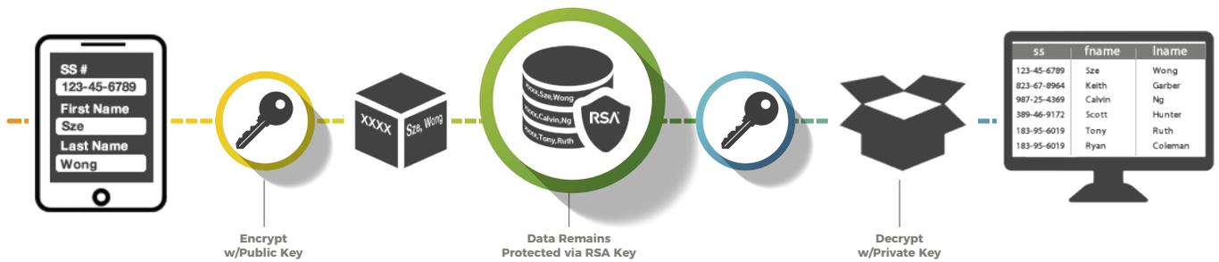
In addition to layers of system-level security, the iFormBuilder platform also offers End-to-End Field-Level Encryption. Users can create a custom public-private key pair to encrypt selected fields. Encrypted fields will be encrypted on the mobile device, through transfer to the cloud and stay encrypted until the data is downloaded to the user's computer. Field-Level Encryption allows iFormBuilder to be approved for use in HIPAA-compliant projects.
